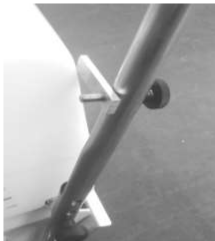
Tank lock in the closed position
